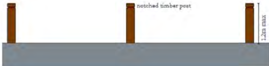
Figure 13 - Fencing Detail 3 - Public Open Space - Conservation
